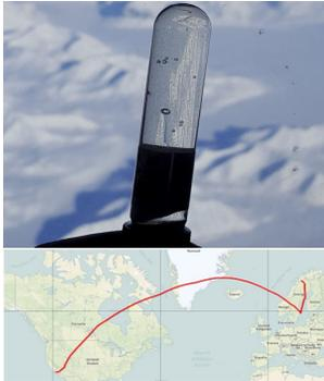
Above: A neutron bubble chamber in an airplane 35,000 feet above Greenland. Spaceweather.com and the students of Earth to Sky Calculus are flying these sensors to measure aviation radiation during solar minimum.
