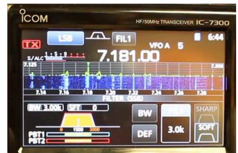
*PBT 1 & 2 (USB/LSB) can be seen graphically on-screen for easy adjustment (lower left)*
