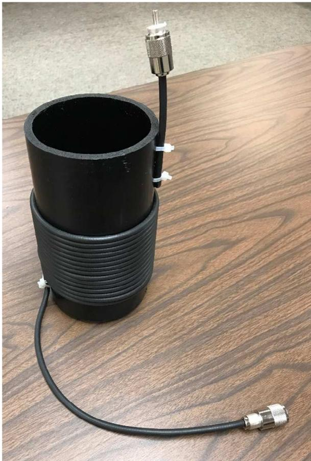
on this PVC pipe. Doing so is necessary in order to achieve an inductance of 50 to 100 uH. Doing so maintains a proper choking of extraneous RF energy that can
